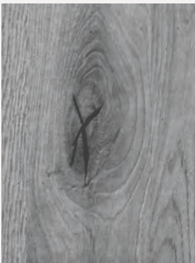
FK / FILLED KNOTS The knots are filled and the wood is planned and sanded to achieve a smooth surface. Only for OAK and not possible on legs.
